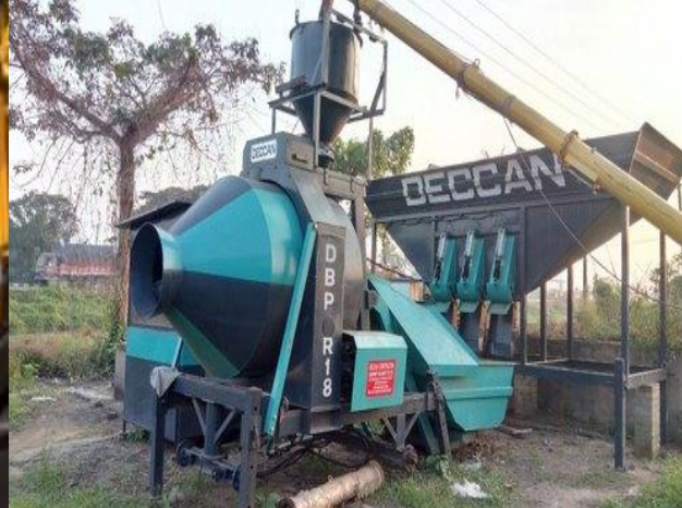
BATCHING PLANT -02 NOS
